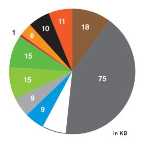
extensions for GP (c15dot4) Zigbee 2015 core stack (c7b) Zigbee Foundation Core (included in c7bfx) Sample set of standard clusters used in this project: Basic, Groups, Identify, Level Control, On/off, Scenes, Thermostat (just a stub that receives temperature reports from GP or Zigbee temperature sensors)
