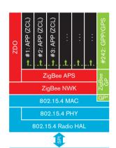
Zigbee Gateway – Embedded Stack Solution
