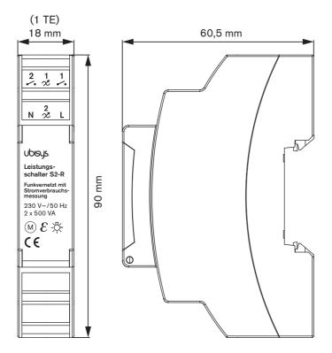
Figure 2: Rail-mount ZigBee Dual Power Switch S2-R - Dimensions
