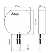
When connecting the Router R0 the included push-wire terminals can be used. Please be aware of the general risks when working on the mains power supply, while installing the component!
