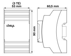
Figure 2. H10/230-XI Wired 230V~/50Hz, H10/24-XI Wired 24V Thermostat Interface Extension Modules – Dimensions
