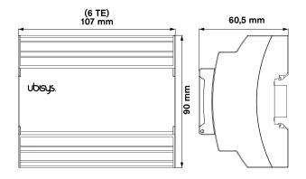
Figure 1. H10/230V-24V-B 10-Channel Zigbee Thermostat for 230V~/50Hz-24V Base Modules – Dimensions
