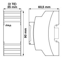
Figure 3. H10-XP Circulation Pump Control, H10-XS Heating/Cooling Demand, H10-XW 1-Wire® Bridge Extension Modules – Dimensions
