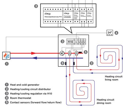
By way of example, a 2-pipe heating/cooling system is shown here that heats or cools via the heat pump in the heat and cold generator (illustration: heating).
