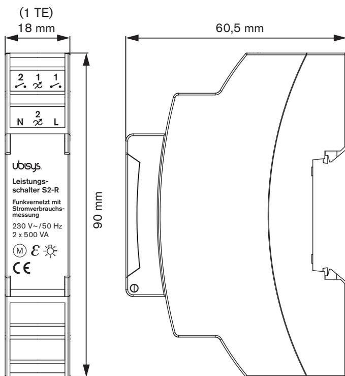
Figure 2: Rail-mount ZigBee Dual Power Switch S2-R – Dimensions
