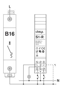
\*) The S1-R has two terminals for the operating voltage (L), which are internally connected. It is not necessary to connect both.
