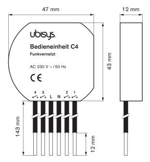
Figure 1: Flush-mount In-wall ZigBee Control Unit C4 - Dimensions
